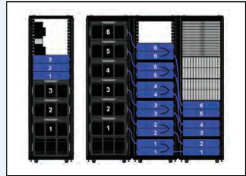
Figure 4. For true modularity and flexibility, look for EBMs that can be placed in the same rack with the UPS, in adjacent racks, daisy chained, and can share space with existing IT equipment.
